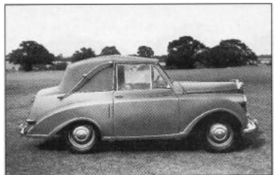
Huge Landau irons dominate side view of Mayflower convertible, semaphore trafficators had to be relocated behind doors
