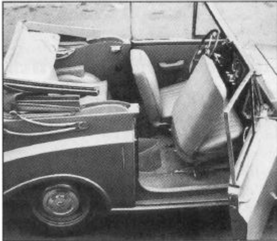
No problem gaining access to rear seat, but stowage of convertible top when lowered was rather ungainly. Removal of saloon roof reduced body rigidity and, despite reinforcement added underneath, this problem was never really cured
