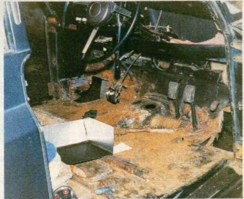
Following advice in manual, Hodgkinsons used apertures in body shell to skewer it and rotate it for easy access to underside. Wings cleaned up, every trace of rust carefully cut away
