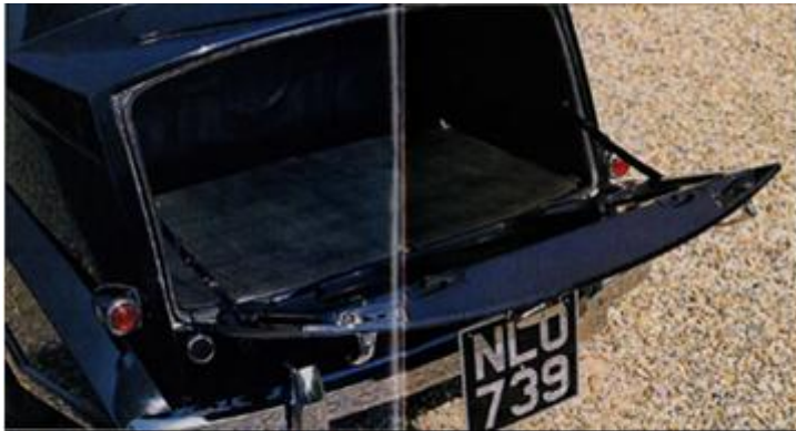
Boot lid can act as load-carrying platform for extra luggage capacity. Note fold down number plate
