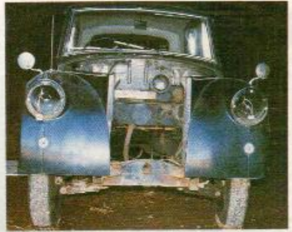
Following advice in manual, Hodgkinsons used apertures in body shell to skewer it and rotate it for easy access to underside. Wings cleaned up, every trace of rust carefully cut away
