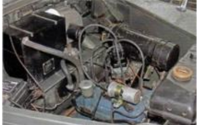
The side valve engine was derived from the pre-war Standard 10. Its 1247cc puts out 38bhp@4200rpm and propels the Mayflower in a quiet and unfussy manner, but not quite all the way up to the 70mph national maximum.
