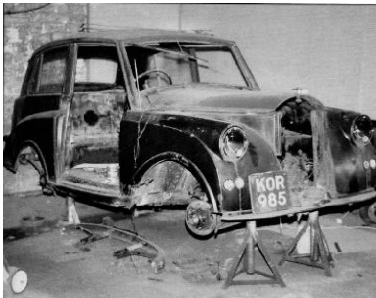
Above, the badly corroded Mayflower shell, completely stripped Left, Alan works on the engine block after forcing out the seized pistons Bottom left, many of the components of the low-mileage engine were reusable Below, the interior was home-trimmed to a very high standard
