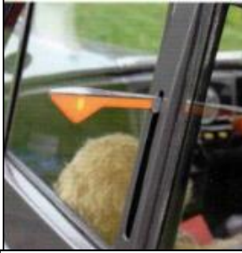
Trafficators are a period curiosity now and flashing indicators are a must.
