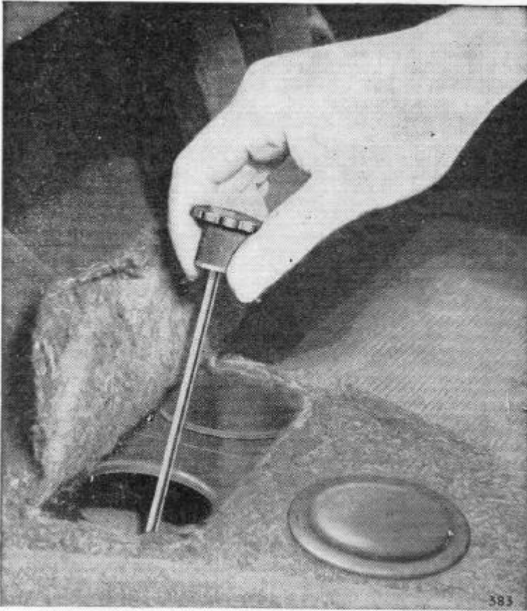
Fig. 10. Gearbox oil filler and dipstick.
