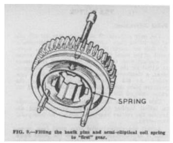
Fit the three baulk pins and semi-elliptical coil spring to the reverse gear. Install this assembly on the mainshaft, afterwards fitting the first speed cup, noting the splines engaged by its three lugs.
