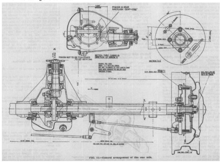
Reassembly of these parts is approximately the reverse of the procedure given above with the necessity to drive or press the bearings on to the shafts. In the absence of a press, a special sleeve tool may be used with a hammer to drive on the bearings.
