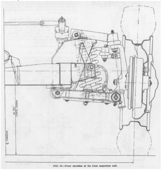
Disconnect the steering outer tie rod from the steering lever.
