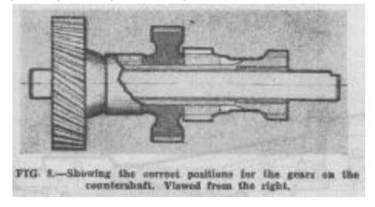
Before fitting new thrust washers gauge check them. The correct end float for the countershaft gears should be between .006 to .010. If there is insufficient end float, the distance collar should be reduced as necessary by rubbing this down on a piece of emery cloth placed on a surface plate. Where too much end float exists, new thrust washers and or distance piece should be fitted.
