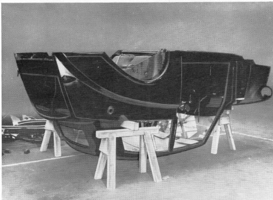
Fig. 5. Showing method of supporting the inverted body on four trestles.
