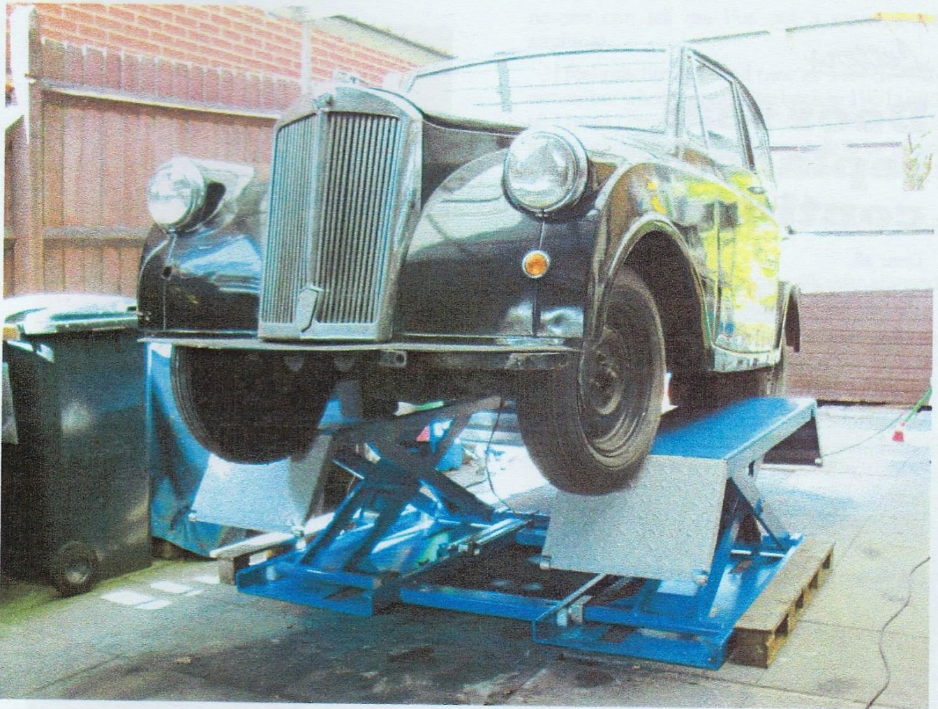
The Triumph Mayflower on the ramps. The lift is at about half height. In this picture it can be seen that the front wheels are just on the edge of the lifting platform.
