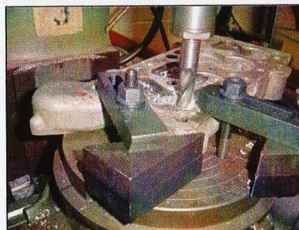
Milling the combustion chamber showing the rotary table.
